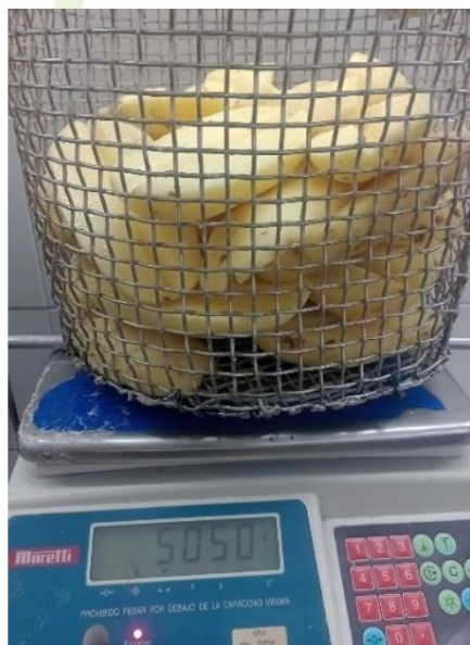
Figure 5. Left: Basket balance for weighing the sample in air and water. Right:
